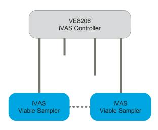
A single cable carries both RS485 communications and 24Vdc power to each iVAS. The connection is via a guick release connector on the free-standing pedestal unit or via a cable rising through the mounting column in the tri-clamp variant. This ensures fast and straightforward iVAS swap outs.
